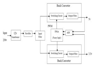
Fig.1 Block diagram of digital controlled SMPS
